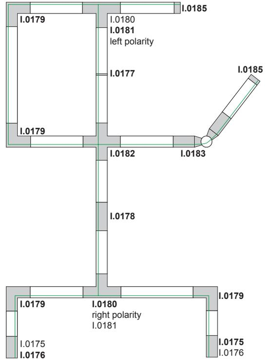
Track is polarized and is manufactured with identifying ridge (green line on diagrams). Refer to these diagrams to ensure proper connector selection.
