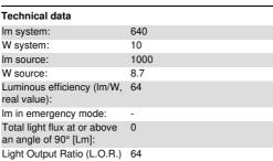
Total light flux at or above an angle of 90° [Lm]: Light Output Ratio (L.O.R.) 64 [%]: Beam angle [°]: 14° CRI (minimum): 80 Colour temperature [K]: 3000 Life Time LED 1: > 50,000h - L80 - B10 (Ta 25°C) Ballast losses [W]: Lamp code: LED
