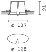
**Product code**MD92: recessed luminaire Ø 137 - neutral white passive dissipation integrated electronic control gear - flood **Attention! Code no longer in production****Technical description**
