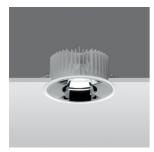
MB69: Round recessed luminaire - D=226 mm H=103 mm - LED warm white - electronic ballast - optic with asymmetrical double emission Attention! Code no longer in production
