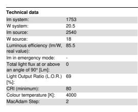
Life Time LED 1: > 50,000h - L90 - B10 (Ta 25°C) Lamp code: LED Number of lamps for optical 1 assembly: ZVEI Code: LED Number of optical assemblies: Power factor: See installation instructions Inrush current:  $5 A / 50 \mu s$ Maximum number of luminaires of this type per miniature circuit breaker: B10A: 31 luminaires B16A: 50 luminaires C10A: 52 luminaires C16A: 85 luminaires Overvoltage protection: 4kV Common mode & 2kV Differential mode DALI-2 Control:
